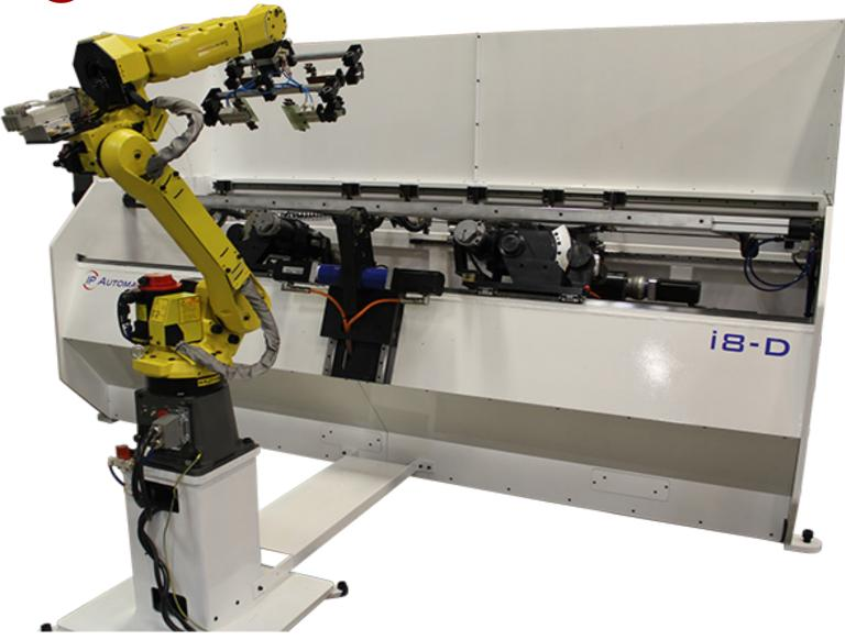
CNC DUAL HEAD WIRE BENDING MACHINE
